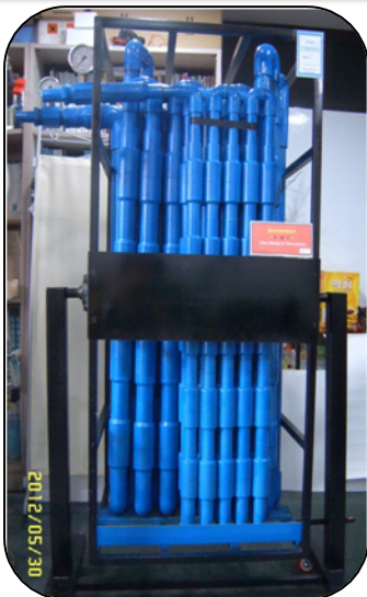
PMF(Pipe Mixer and Flocculator) W500 x L500 x H1500(He 1200)
